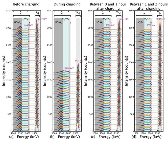
**Figure 1.** Energy spectra obtained consecutively for an acquisition time of 1 min: a) for 1 h before charging, b) during charging, c) for 1 h immediately after charging, and d) between 1 and 2 h after charging. An off-set is applied to distinguish the various spectra and the different regions of the battery are indicated.
