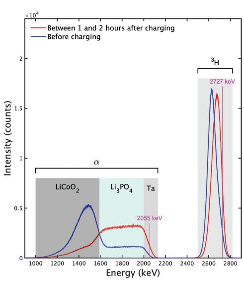
Figure 3. Comparative energy spectra obtained for an acquisition time 1 h. The blue and red curves show the spectra obtained for 1 h before charging and between 1 and 2 h after charging, respectively.
