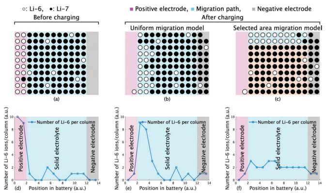
**Figure 7.** Migration path models in the  $Li_3PO_4$  solid electrolyte. a) Initial (before charging) distribution of lithium-6 and lithium-7 ions (atoms), b) distribution of lithium-6 and lithium-7 ions (atoms) in the final state (after charging) when migrated by the uniform migration model, c) equivalent distribution for the selected area migration model. d–f) represent, respectively, changes in the number of lithium-6 ions as a function of position (column) in (a)–(c).
