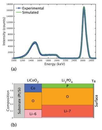
**Figure 5.** a) Analysis of energy spectra before charging using SIMNRA. b) Schematic of the depth profile of each element of each layer.
