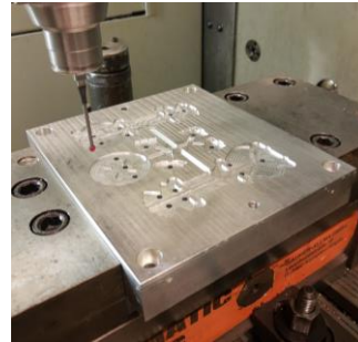
b) CNC milling of the moulds
