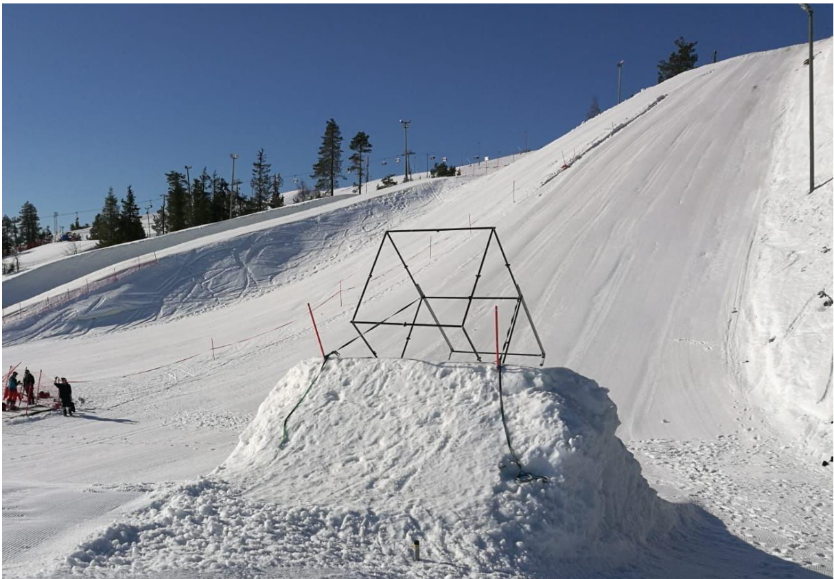
FIGURE 1. Calibration cube was set on the peak of the jumper with the help of load straps.
