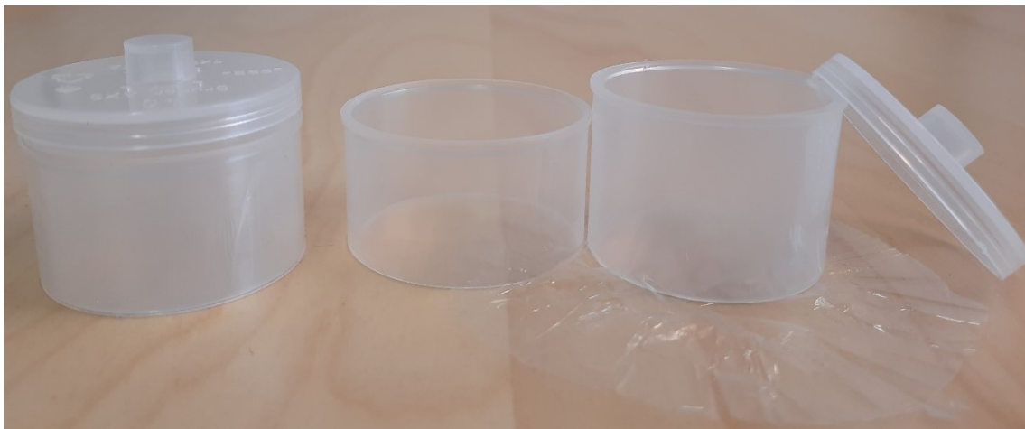
Figure 13 Liquid sample cup accessories (right) and one prepared cup (left).
