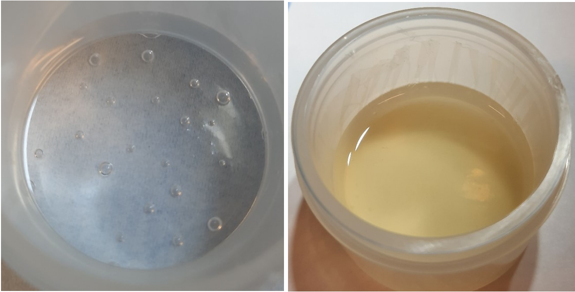
Figure 26 Bubble formation in standard solution (left) and wastewater sample (right).
