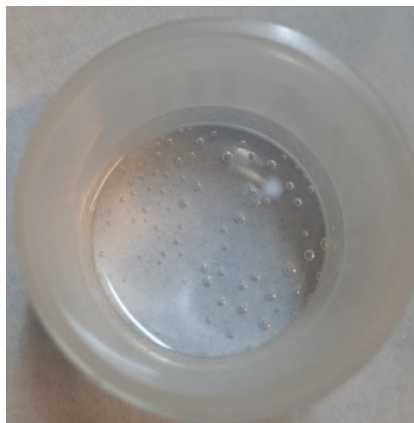
Figure 22 Bubbles at the bottom of the measurement cup.
