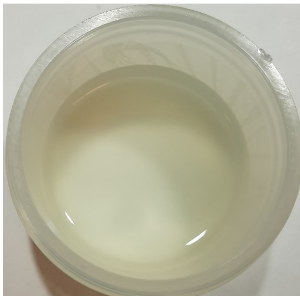
Figure 28 Standard solution with 0.05% Triton X-100 after XRF measurement.
