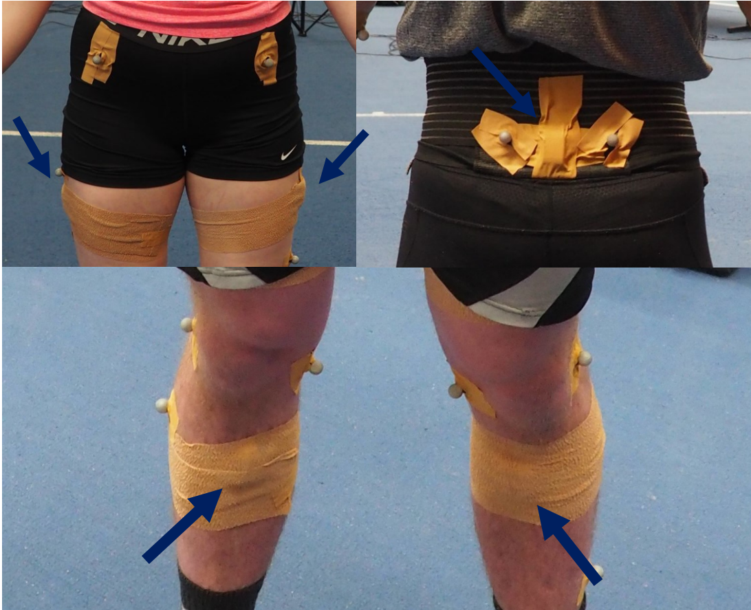
FIGURE 14. The placement of the thigh, shank, and pelvis IMUs (IMU locations shown with blue arrows). All IMUs were located x-axis vertically (upwards positive), and y-axis to the left on the surface.
