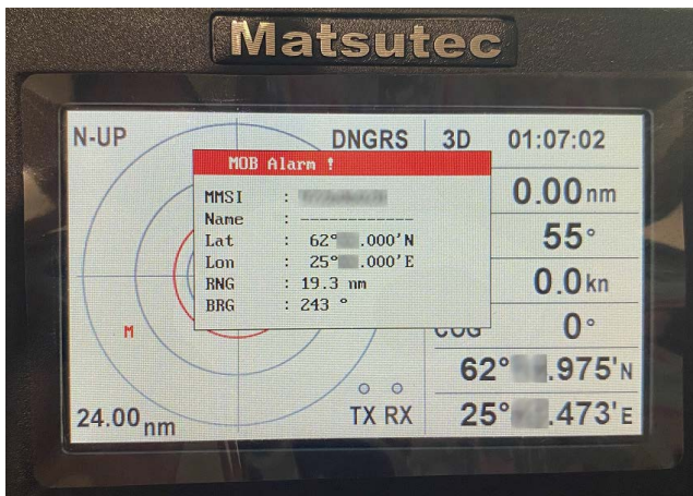
FIGURE 6. MOB alert in the Matsutec HP-33A AIS transponder.
