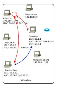
Fig. 1. Simulation Laboratory architecture presenting ARP poisoning.
