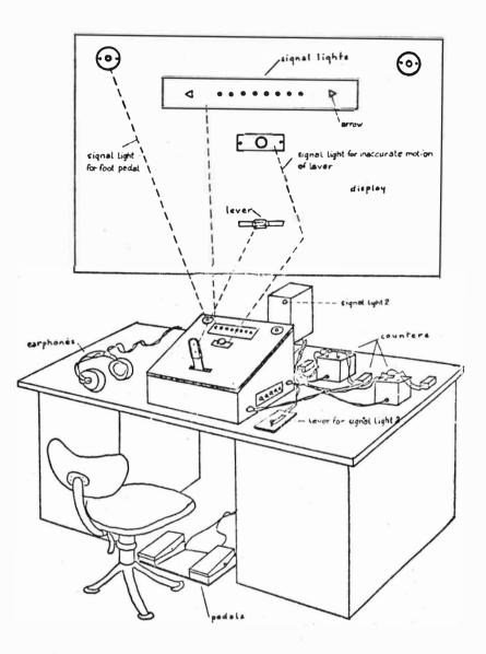
Figure I. Choice reaction test equipment
