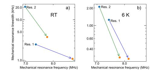
**Figure 3.** Plots of the resonators' mechanical resonance frequencies and linewidths before (blue) and after (orange) the annealing at room temperature (a) and 6 K (b). The values before and after annealing have been connected with blue (resonator 1) and green (resonator 2) arrows for clarity.
