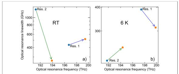
**Figure 4.** Plots of the resonators' optical resonance frequencies and linewidths before (blue) and after (orange) the annealing at room temperature (a) and 6 K (b). The values before and after annealing have been connected with blue (resonator 1) and green (resonator 2) arrows for clarity.
