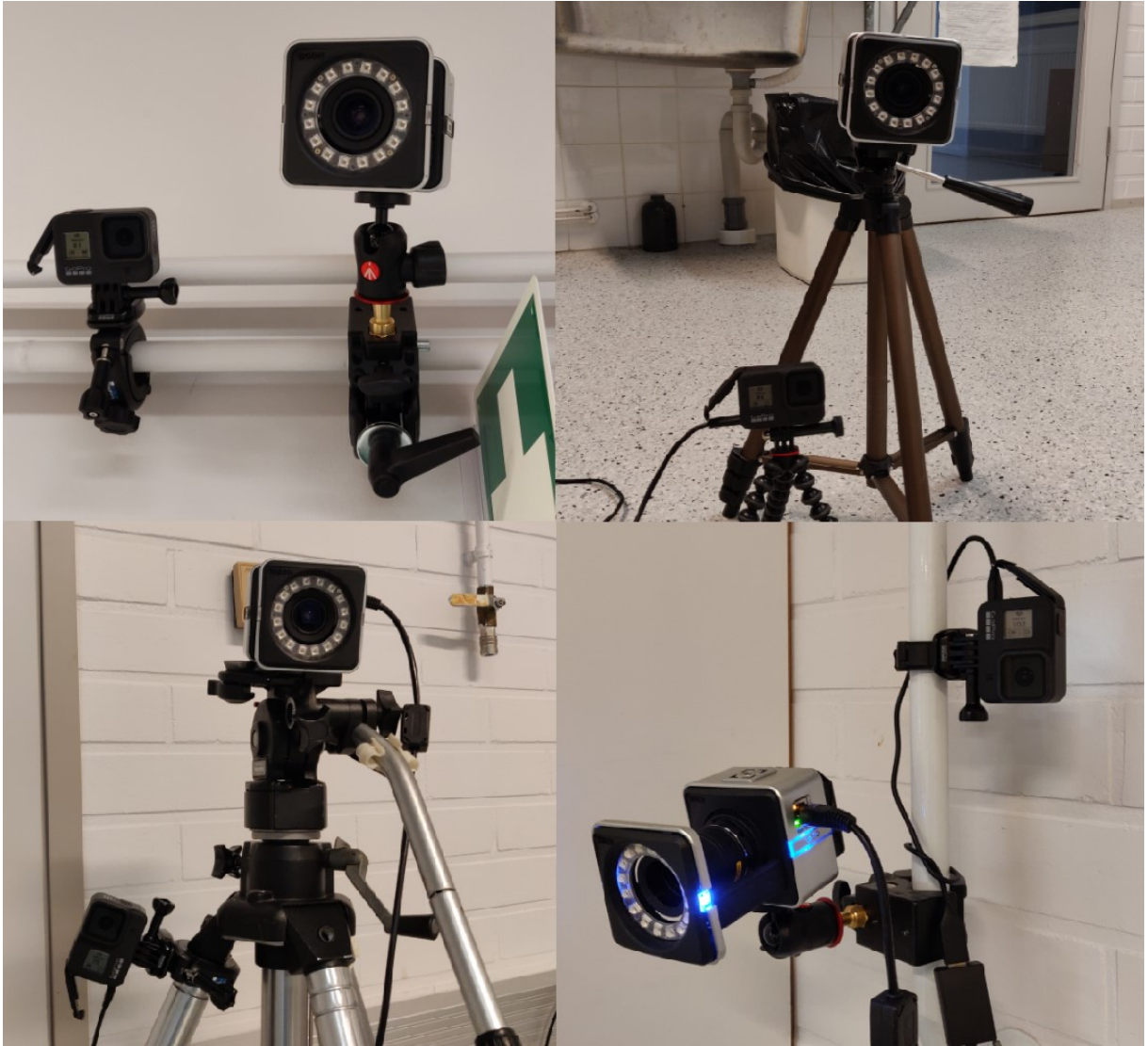
FIGURE 18. Examples of camera attachments and relative locations of cameras in a pair. Distances between cameras in a pair varied from 15 to 30 cm.
