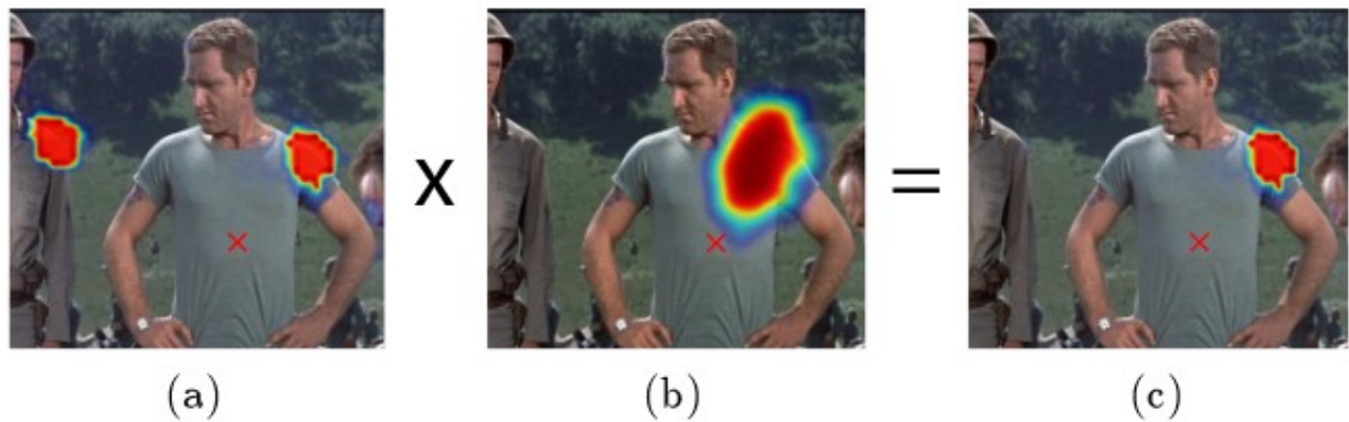
FIGURE 11. Spatial model implemented in Jain et al. (2014) for masking out the incorrect joint heatmaps. A joint mask (b) is used to describe the possible joint locations when the torso is centered in the mask. In (a) there are two separate heatmaps for left shoulder from which the incorrect one is masked out in (c).
