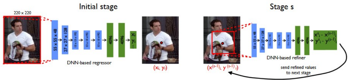
FIGURE 10. Schematic view of the 2D HPE process of DeepPose (Toshev & Szegedy 2014). The network makes an initial estimation of the joint location from a down-sampled input image (left). In stage s , the network refines the initial estimation from a cropped higher-resolution input image.
