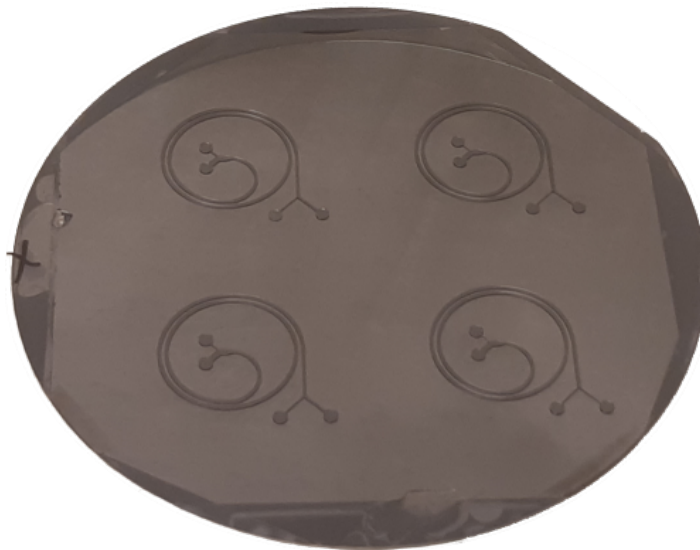
Figure 10. Mould used for PDMS chips. It is made with negative photoresist SU-8 on a silicon wafer. It features the spiral design of the channels, in reverse.
