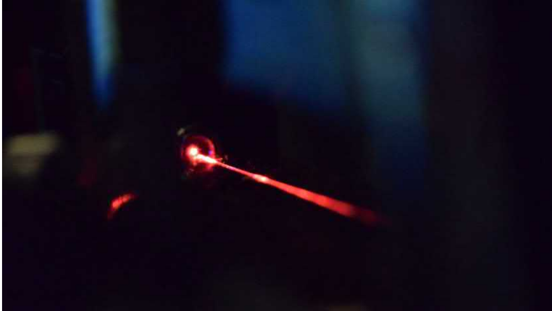
Fig. 5.4. Photonic-crystal fiber, generating red light via continuous broadening from IR. Infrared light with a spectrum centered at 1050 nm (see Fig. 4.10 (b)) enters the SC-975 fiber from the bottom right-hand corner in the picture, and red light is gradually generated via SPM. Note that SPM broadens the spectrum continuously and symmetrically, so that also longer wavelength IR light is generated. A collimating lens (L3) can be seen by the fiber end.
