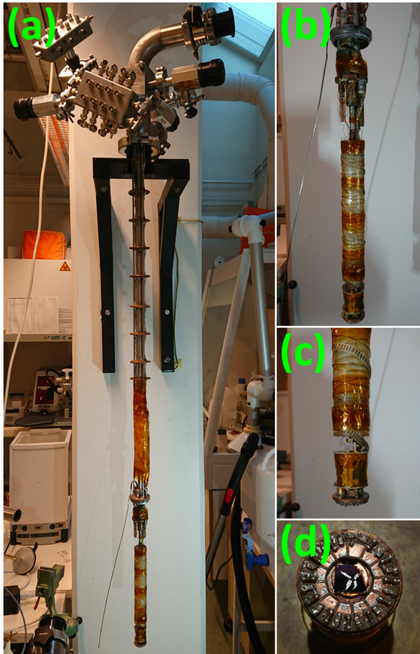
FIGURE 27 The in-house built ^3\text{He}/^4\text{He} dilution refrigerator. (a) The full cryostat with pump and measurement line connections on the top. (b) A zoomed-in picture of the bottom part, which contains the main functioning parts of the cryostat including the pot, the still and the mixing chamber. (c) A closer view of the mixing chamber and the stage holder. (d) Sample mounted onto the sample stage. The sample connections were made with indium bonding and thus large indium joints are visible
