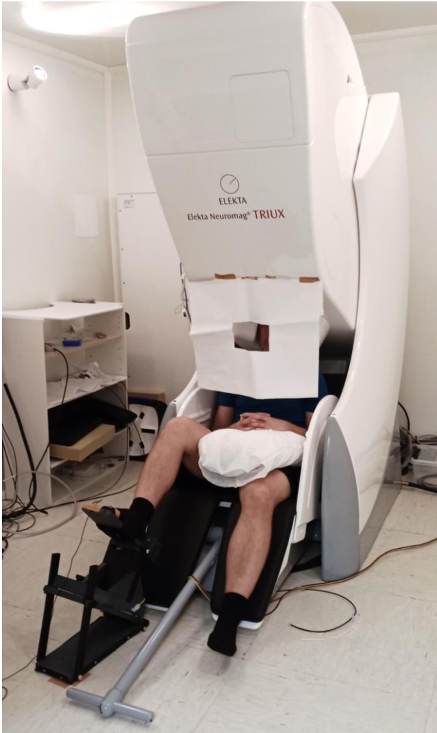
FIGURE 9. Setup of CKC protocol in magnetically shield room. Subject's dominant leg is attached to ankle actuator. Auditory interferences are blocked with ear plugs and brown noise auditory track and visual interferences of leg movement are covered with white paper.
