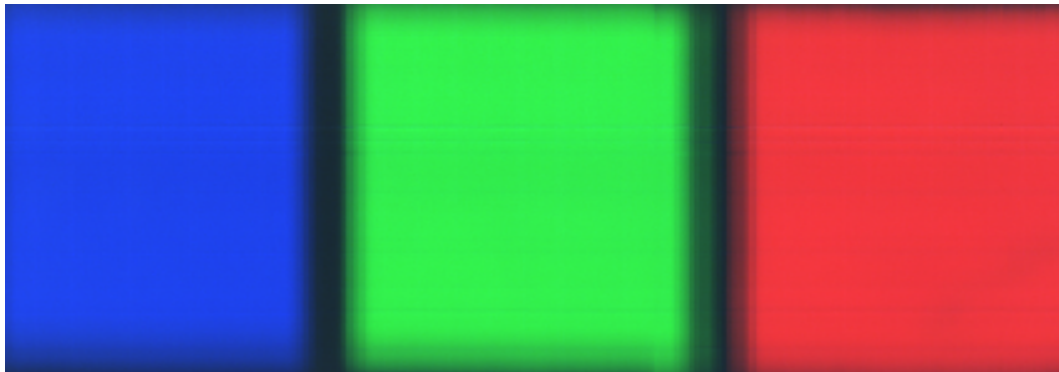
Figure 7. False color image constructed from the scan of the color checker. Scanning direction was from right to left. Blurry edges between the color tile boundaries are caused by uneven scanning speed of the manually driven scan. Vertical shift in the green tile is due to losing connection to the desk during the scan.
