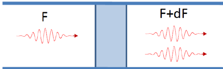
Figure 2.2. Elementary change dF in the photon flux F during the dissemination of a plane wave from the material.
