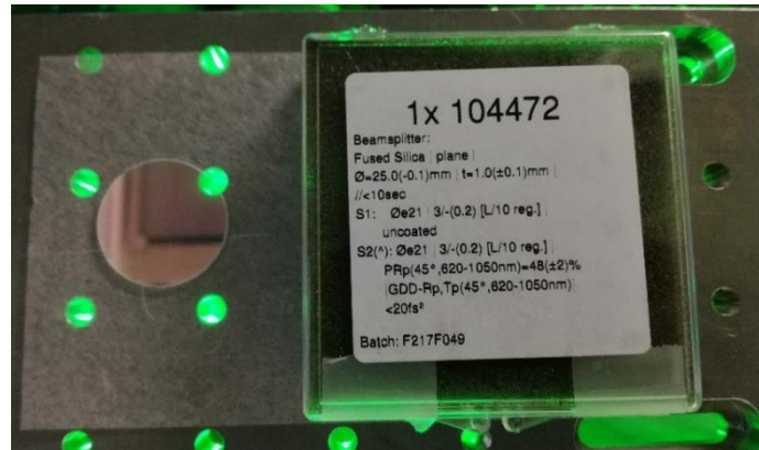
Figure 4.6. Partially reflecting mirror with reflectivity of 48%.
