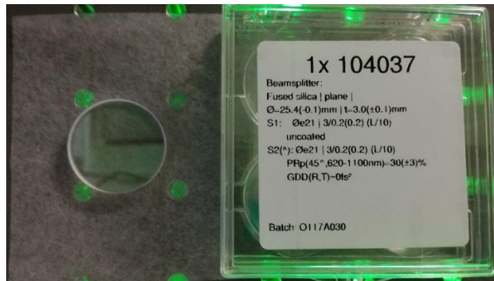
Figure 4.4. Partially reflecting mirror with 30% reflectivity.
