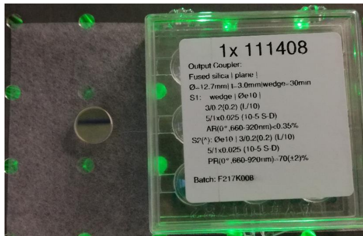
Figure 4.9. Partially reflecting mirror with 70% reflectivity.
