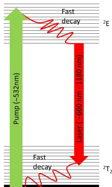
Figure 2.5. Ti:sapphire structure of energy levels [2].
