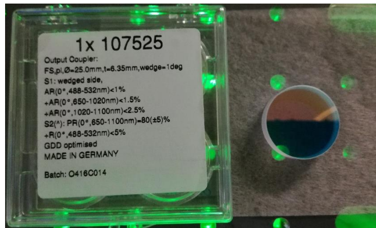
Figure 4.10. Partially reflecting mirror with reflectivity of 80%.
