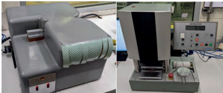
Figure 7.18 RCT & Concora Tester from Lorentzen & Wettre Products (now ABB).
