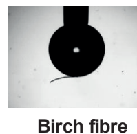
Figure 3.23a) Bubbles on the model surfaces of cellulose, TMSC and CNF in water. Only on TMSC bubbles showed clear attachment. b) Birch fiber attached on a bubble.
