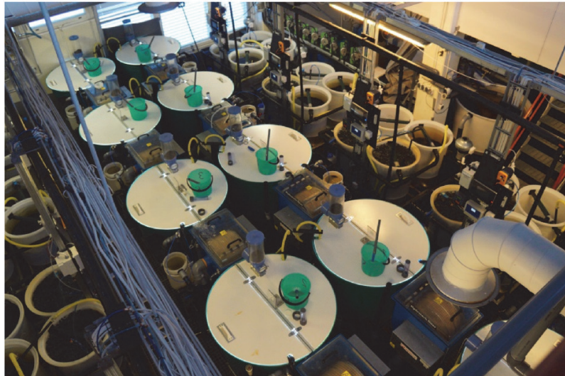
Fig. 1. RAS platform built in Natural Resources Institute Finland (Luke) Laukaa fish farm.
