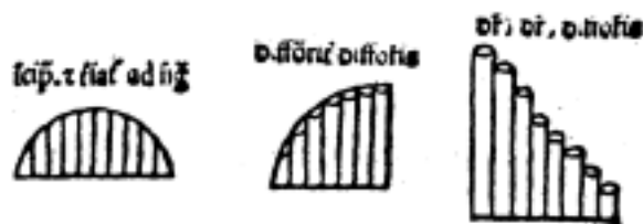
Figure 1.1 – Oresme’s diagram of latitude and longitude, representing the change of velocity (the vertical bars) against time, from The Latitude of Forms (Oresme, 1968).
