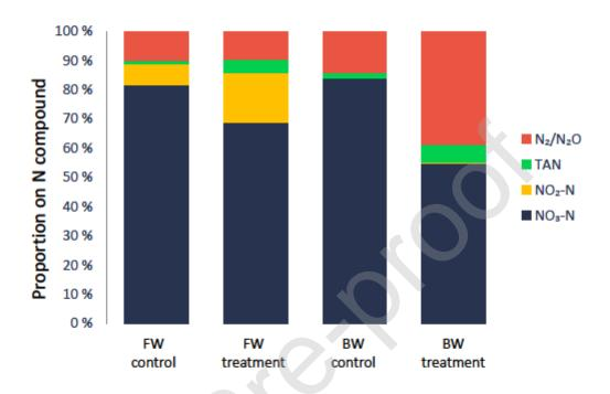
**Figure 4.** Average percentages of different N compounds in the outflows of woodchip bioreactors fed with freshwater (FW) and brackish water (BW) RAS overflow discharge (Control) or RAS overflow discharge with supernatant from the sludge coagulation (polyaluminum chloride) and flocculation process (PrimeBOND A0415 and PrimePHASE; Treatment) during the six weeks study. Woodchip reactors were run in duplicates.
