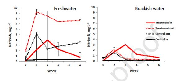
**Figure 5**. Nitrite-nitrogen ( $NO_2$ -N) in the inlet and outlet of woodchip bioreactors fed with freshwater (Figure A) and brackish water (Figure B) RAS overflow discharge (Control) or RAS overflow discharge with supernatant from the sludge coagulation (polyaluminum chloride) and flocculation process (PrimeBOND A0415 and PrimePHASE; Treatment) during the six weeks study. Data is mean  $\pm$  SD, n=2.
