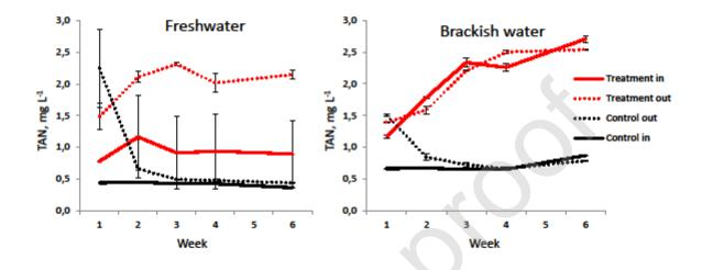
**Figure 3**. Total ammonia nitrogen (TAN) in the inlet and outlet of woodchip bioreactors fed with freshwater (Figure A) and brackish water (Figure B) RAS overflow discharge (Control) or RAS overflow discharge with supernatant from the sludge coagulation (polyaluminum chloride) and flocculation process (PrimeBOND A0415 and PrimePHASE; Treatment) during the six weeks study. Data is mean  $\pm$  SD, n=2.
