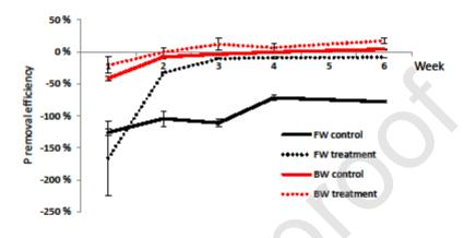
**Figure 2**. Phosphate-P removal in the woodchip bioreactors fed with freshwater (FW) and brackish water (BW) RAS overflow discharge (Control) or RAS overflow discharge with supernatant from the sludge coagulation (polyaluminum chloride) and flocculation process (PrimeBOND A0415 and PrimePHASE; Treatment) during the six weeks study. Data is mean  $\pm$  SD, n=2.
