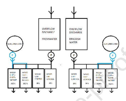
**Figure 1**. Schematic diagram of the experimental set-up. P = peristaltic pump.
