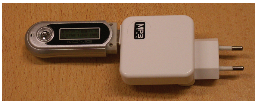
Fig. 2. MP3 player with an embedded FM transmitter, connected to power adapter. The antenna is not connected.
