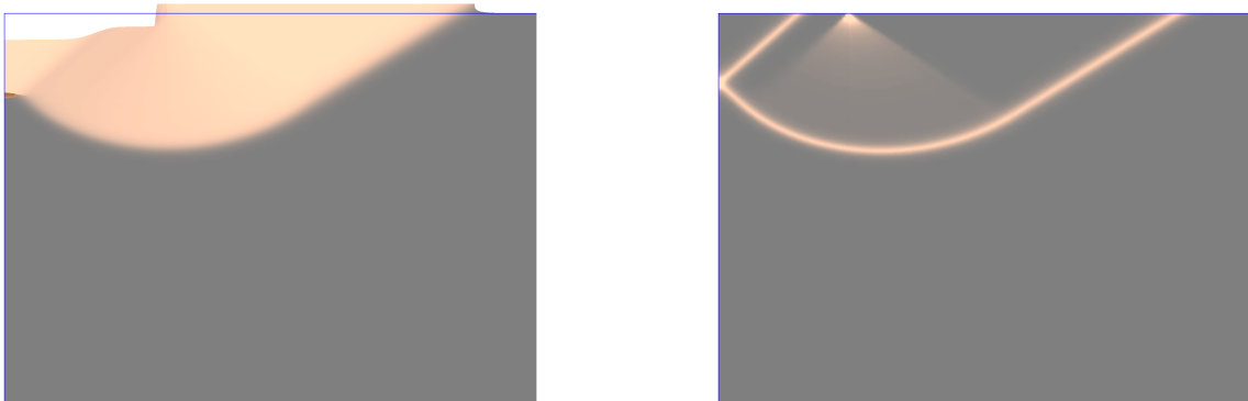
Figure 6: The field u_{h, \alpha_{\max}} with enlarged deformed shapes (left) and the divergence of u_{h, \alpha_{\max}} (right) for the finest mesh – strip footing problem.
