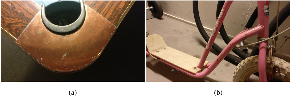
Figure 1: Figure (a) shows a metal-coated pool table pocket with impact marks. The coating has been almost completely worn off from the edges and corners. Figure (b) shows how easily accessible outer parts of the kick scooter's frame have suffered a lot of impacts. Coating penetration has caused rust to appear.
