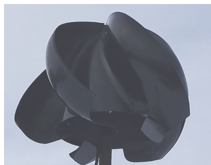
FIGURE 52. Small wind generator for the roof of a house (0.3 kW, 1kW or 2 kW,...).
