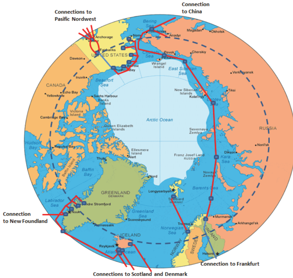
FIGURE 41. The Arctic region undersea optical cable systems now and in the near future (PII, PIII and PV).
