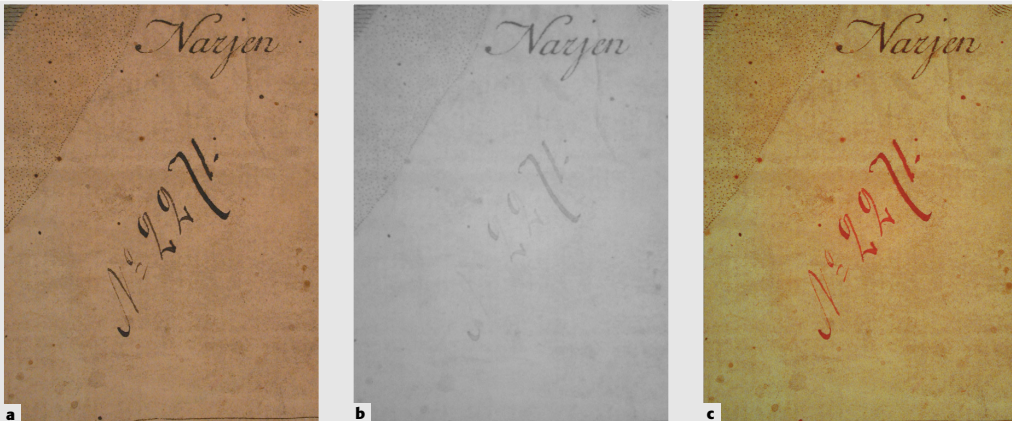
6 Examples of close up photographs with wide angle not suffering from the hotspotting phenomena: RGB image (a) , IR image (b) , and combined FCIR image (c) . Photographs by paper conservation student Maija Kupari, image processing István Kecskeméti.
