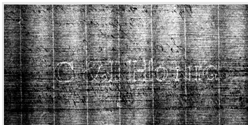
7 The same image as in Fig 6 with high contrast, created in Adobe Photoshop software (Image - Adjust - Brightness/Contrast). This is a more enhanced way of making the watermark more visible. It needs some practice not to overuse the increased contrast.
