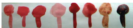
Fig. 5: The inks presented in Fig. 3 in FCIR image. All inks except sepia and bistre show red, which is typical of iron gall inks.
