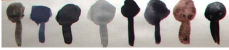
Fig. 2: Akvila ink 152 (fountain pen ink) from the 1940's; Akvila ink 152 (fountain pen ink) from the 1960's; Akvila ink 109 (archival ink) from the 1960's; Akvila ink 109 (archival ink diluted with water from dry powder) from the 1960's; self-made iron gall ink 3; self-made iron gall ink 2; sepia ink from Kremer pigments, bistre ink from Kremer pigments. Unaged. Full colour RGB image.
