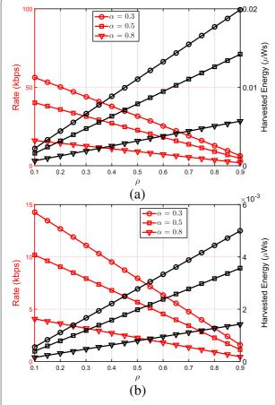
**Fig. 7** Achievable rate and harvested energy versus increasing values of  $\rho$ , where  $\eta=0.3$  and (**a**)  $d_1=d_2=5$ m, (**b**)  $d_1=d_2=10$ m
