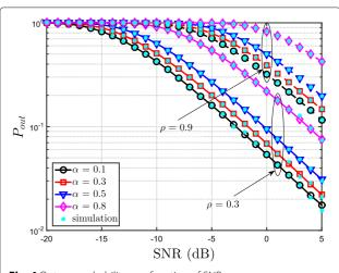
Fig. 4 Outage probability as a function of SNR
