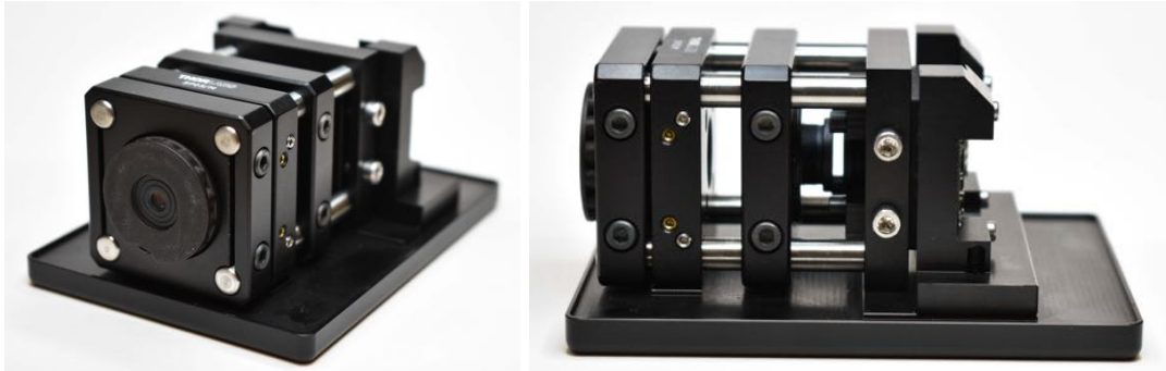
Figure 3: Interchangeable optomechanics mounted to baseplate.
