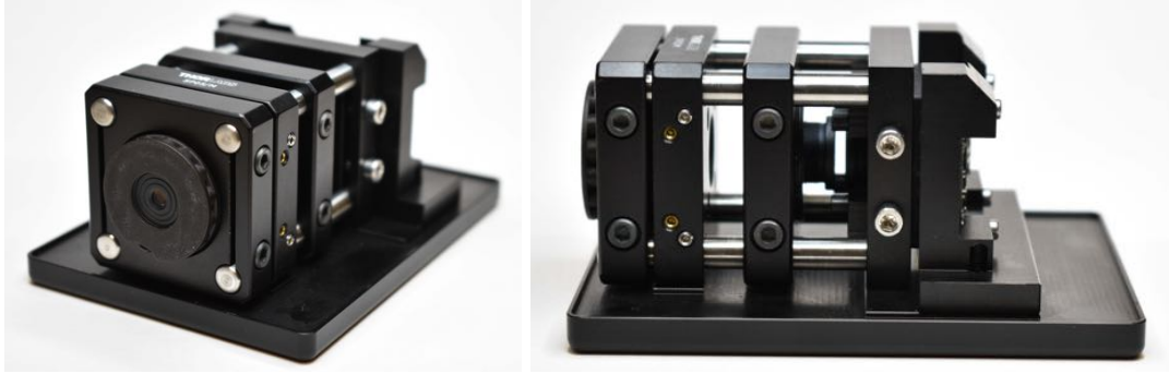
Figure 3: Interchangeable optomechanics mounted to baseplate.
