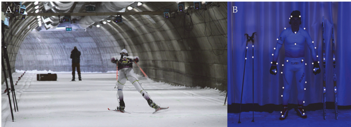
FIGURE 9 Vicon Nexus camera system mounted on Vuokatti ski tunnel and subject skiing with reflective markers as well as ski and pole force measurement systems installed (A). Subject and equipment showing the marker placement during the pilot measurements with one marker missing from both skis (B).
