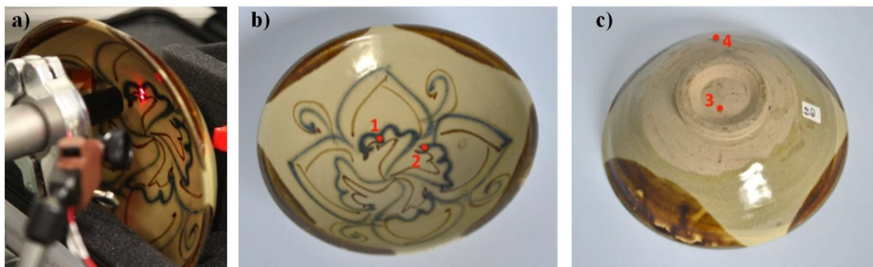
Figure 1. a) PIXE setup of the bowl, b) bluish/greenish measurement positions (1-2) from the front side and c) body clay (3) and thick glaze (4) positions from the back side of the bowl.
