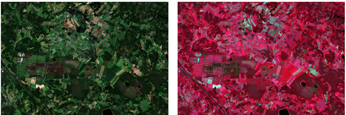
Figure 3. Left: RGB-image composed of red, green and blue bands. Right: False-color infrared -image composed of NIR, red and green bands (Copernicus Sentinel Data[2018], processing: SYKE)
