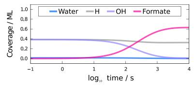
Figure 7: A plot of surface coverages and partial pressures during a microkinetic analysis of the  $\rm ZrO_2$  surface at 700 K with 1:1  $\rm H_2O:CO$  ratio and 2 bar s<sup>-1</sup> flow rate. For the sake of clarity, intermediates whose coverage was < 0.01 monolayers throughout the entirety of the simulation time were not plotted.
