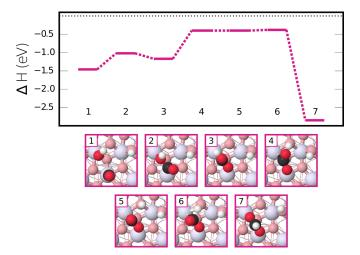
Figure 6: Potential energy diagram and structure geometries for formate formation on  $ZrO_2$ . The gas-phase reference is (H<sub>2</sub>O + CO). Rh, Zr, H, O<sub>ads</sub> and O<sub>lat</sub> atoms are shown in grey, lavender, white, red, and pink, respectively.
