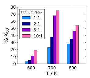
Figure 10: CO conversion, %X<sub>CO</sub>, at the interface at different reaction conditions.
