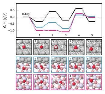
Figure 2: Potential energy diagram and adsorption structures for water adsorption and dissociation on Rh, ZrO<sub>2</sub>, and the Rh/ZrO<sub>2</sub>-interface shown in black, pink, and teal lines, respectively. Rh, Zr, H, O<sub>ads</sub> and O<sub>lat</sub> atoms are shown in grey, lavender, white, red, and pink, respectively.
