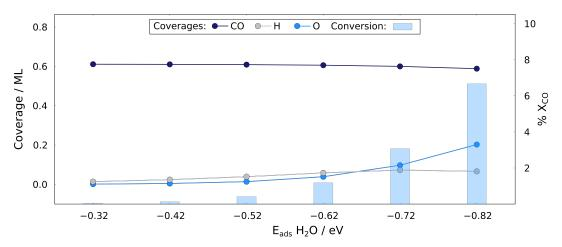
Figure 9: CO, O, and H coverages, and CO conversion,  $\%X_{CO}$ , at steady state WGS plotted against  $H_2O$  adsorption energy. The CO adsorption energy was kept at the original DFT value. Note that the lines connecting the data points are for the purpose of guiding the eye only, and do not indicate interpolation of data. The reaction conditions were kept at 700 K with 1:1  $H_2O$ :CO ratio and 2 bar s<sup>-1</sup> flow rate.
