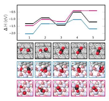
Figure 4: Potential energy diagram and structure geometries for carboxyl formation and dissociation on Rh,  $ZrO_2$ , and the interface shown in black, pink, and teal, respectively. In the cases of Rh and the interface, the gas-phase reference is  $(H_2O - \frac{1}{2}H_2 + CO)$ , but for  $ZrO_2$  it is  $(H_2O + CO)$ , since hydrogen is kept coadsorbed on the surface. Rh, Zr, H,  $O_{ads}$  and  $O_{lat}$  atoms are shown in grey, lavender, white, red, and pink, respectively.
