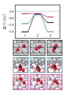
Figure 3: Potential energy diagram and adsorption structures for CO oxidation on Rh,  $ZrO_2$ , and the Rh/ $ZrO_2$ -interface shown in black, pink, and teal, respectively. In the cases of Rh and the interface, the gas-phase reference is ( $H_2O - H_2 + CO$ ), but for  $ZrO_2$  it is ( $H_2O + CO$ ), since hydrogen is kept coadsorbed on the surface. Rh, Zr, H,  $O_{ads}$  and  $O_{lat}$  atoms are shown in grey, lavender, white, red, and pink, respectively.
