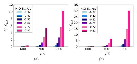
Figure 8: CO conversion,  $\%X_{CO}$ , as a function of temperature with different water adsorption energies, with the CO adsorption energy of a) -1.91 eV, and b), -1.45 eV, which corresponds to our original DFT computed value, and an experimental value, <sup>80</sup> respectively. The inlet gas composition was kept as 1:1 H<sub>2</sub>O:CO with 2 bar s<sup>-1</sup> flow rate. Note the different ranges of the y-axes.
