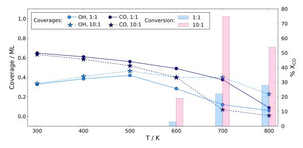
Figure 11: OH and CO coverages, and CO conversion,  $\%X_{CO}$ , at steady state WGS plotted against temperature under 1:1 and 10:1 H<sub>2</sub>O:CO ratio. Note that the lines connecting the data points are for the purpose of guiding the eye only, and do not indicate interpolation of data.
