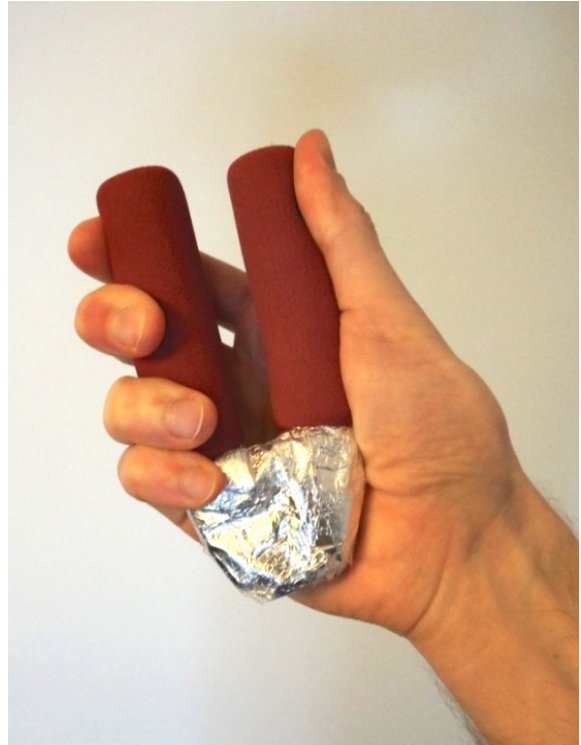
Figure 5. The gripper used in the static gripping task. Gripper's metal part was covered with aluminium foil to prevent disturbances to the MEG device.
