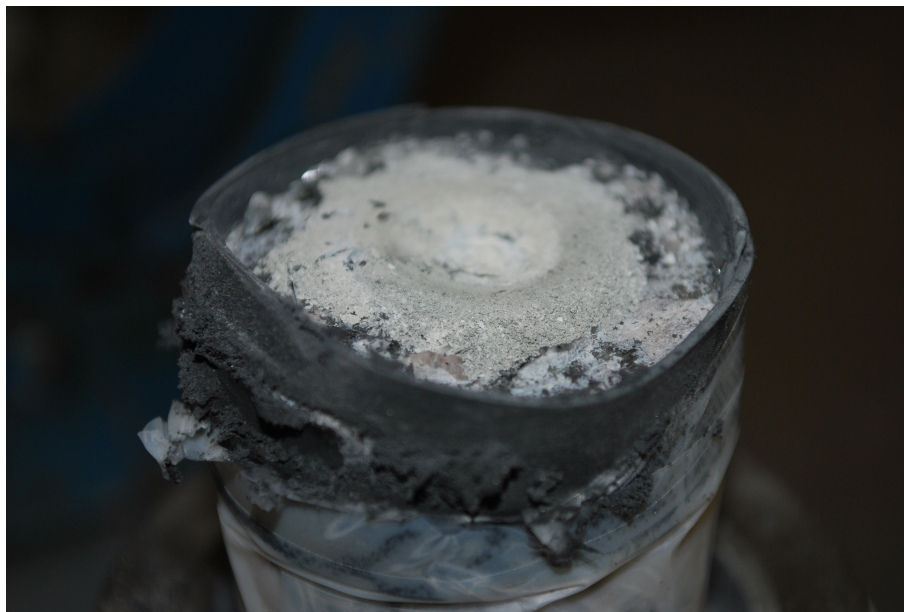
Figure 30. Black plastic collar ground against the surface of the upper rock sample.
