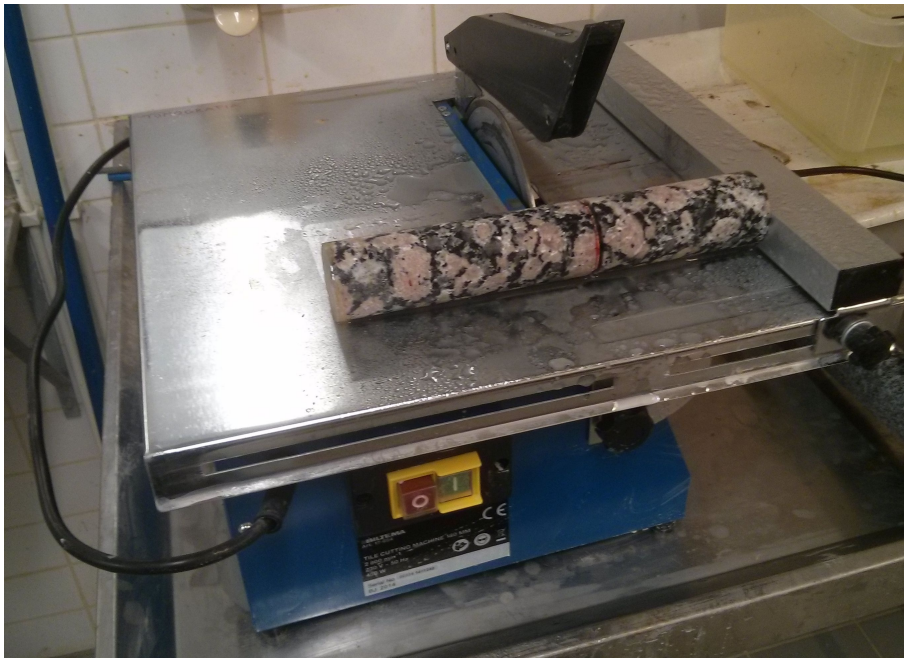
Figure 20. The cutter used to manufacture the samples.
