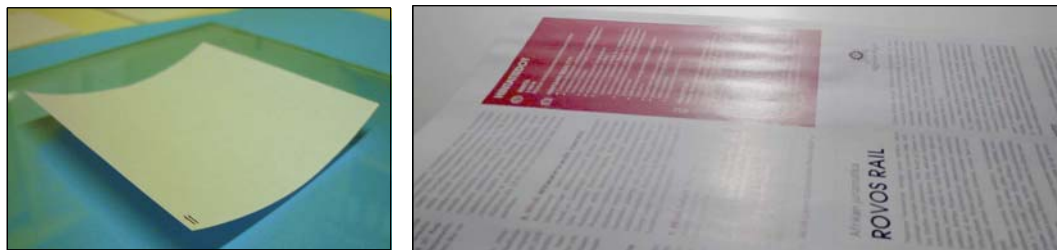
Figure 1: Examples of out-of-plane deformations of paper: picture of fine paper curl (left) and fluting in a printed area of a HSWO printed product (right).
