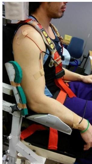
FIGURE 12 – The Electrode Placement. An electrode was placed at the biceps brachii level, while the other was placed in proximity of the scapular bone. Lastly, a reference electrode was placed on the wrist bone.
