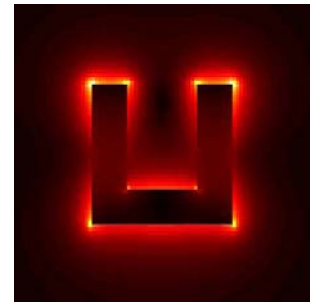
Figure 1: Electric field amplitude in a gold split-ring resonator.
