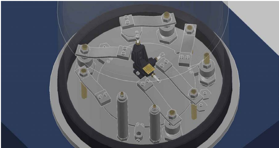
Fig.1. AutoCAD design of the Helsinki TCT vacuum chamber including the sample holder.
