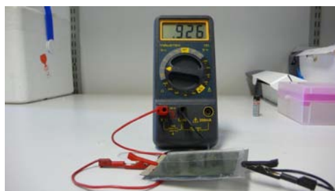
Figure 1. Open circuit voltage of the fresh Pani-aluminum battery is typically between 0.9 – 1.0 Volts.
