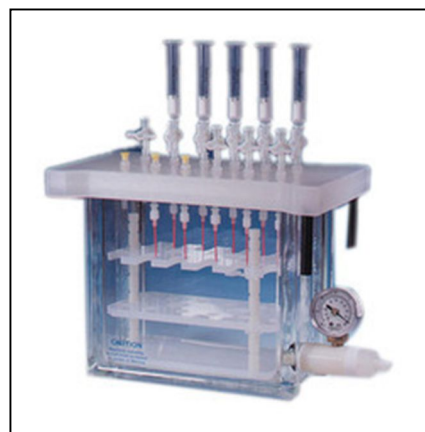
Figure 25. Phenomenex SPE teflon vacuum manifold /83/.
