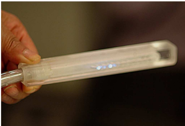
FIGURE 12. One of the optical cable light bars used to visualize the torque level and rhythm.
