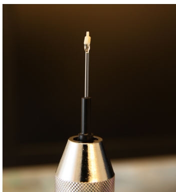
Figure 8.4: A sample of human cortical bone glued on a glass capillary ready for \mu CT imaging.
