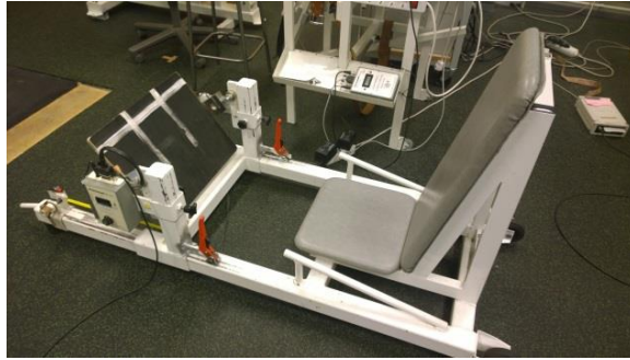
FIGURE 12. The isometric leg press used in evaluation of isometric strength of leg extensor muscles.
