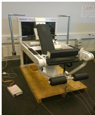
FIGURE 13. The modified David 200 used for isometric knee extension and isometric knee flexion.
