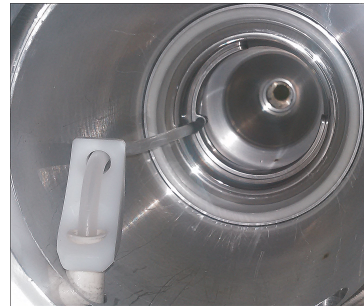
(b) The HV barrier with a cable guide.
