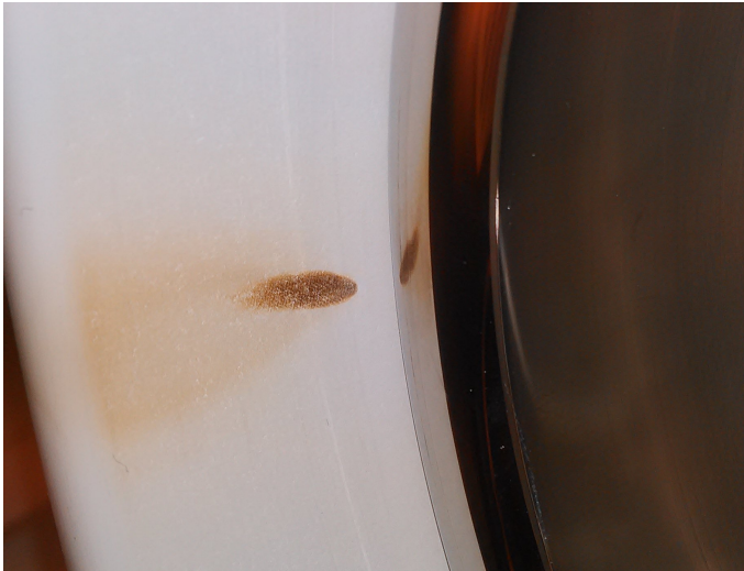
Figure 3.30: The downstream edge of the original HV barrier showing damage from excessive sparking.
