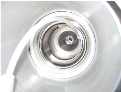
(a) The HV barrier installed as originally planned.
