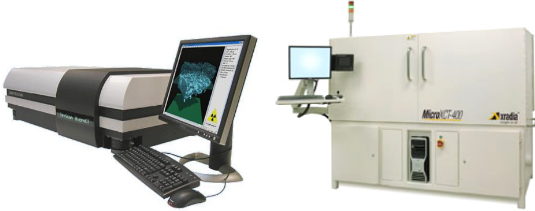
Figure 3.1: The X-ray tomography devices used in the work, SkyScan 1172 (left panel) and Xradia MicroXCT-400 (right panel).
