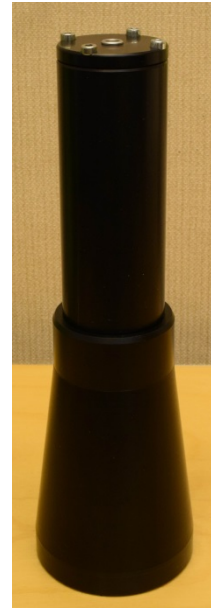
Fig. 4.7 Photo of the LED calibration system.
