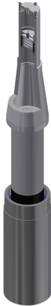
Fig. 4.6 Cut view of the LED calibration system attached to the PMT (3D model).
