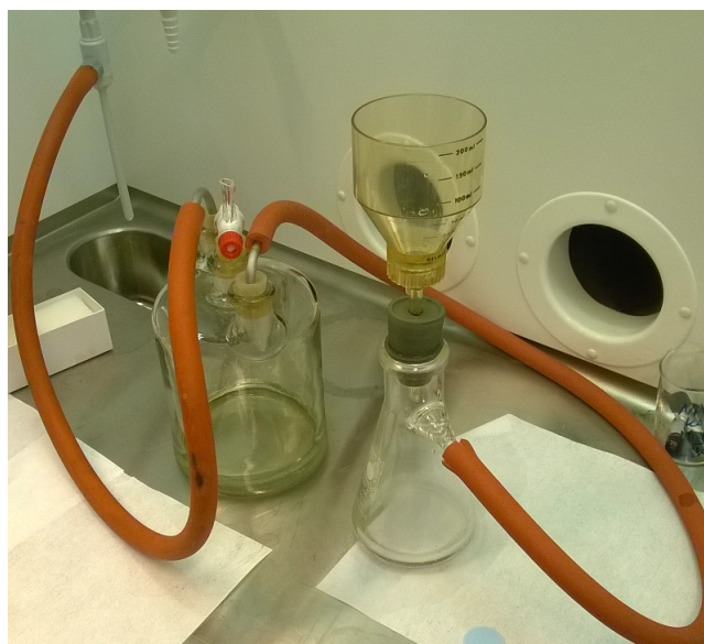
Figure 19: Photograph of the actual vacuum filtration setup.
