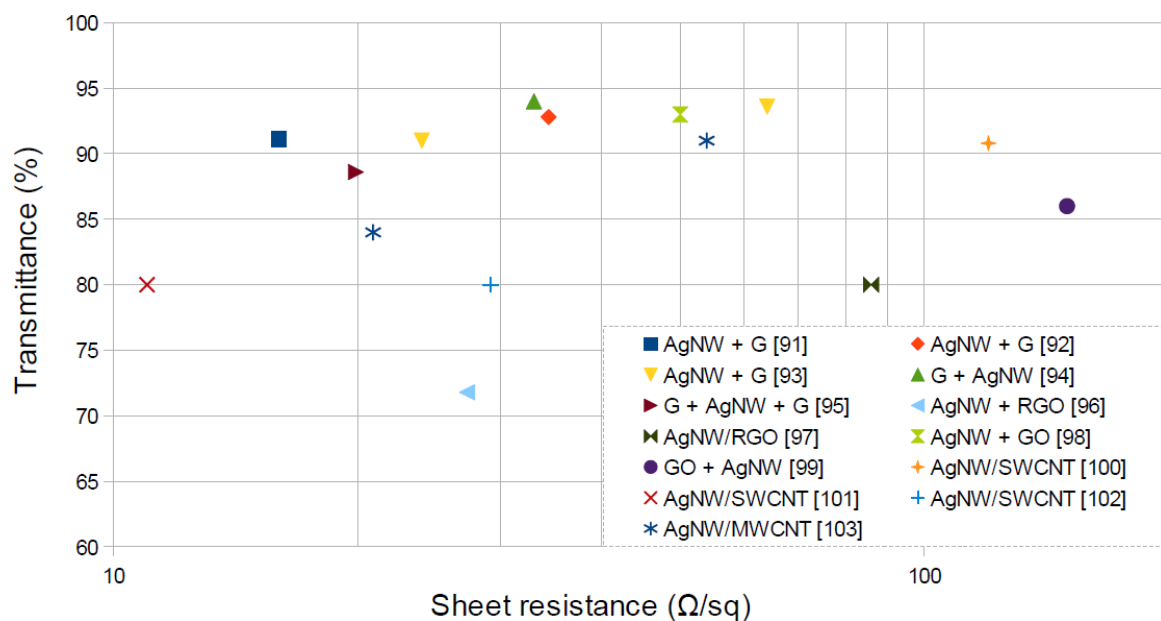
Figure 12: Transmittances and sheet resistances of silver nanowire and carbon hybrid films with the different layers given in their order of deposition starting from bottom or with / in case of mixtures. G refers to CVD grown and directly transferred graphene.
