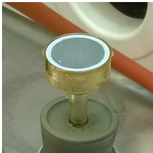
Figure 20: Photograph of the HC-DWCNT film after filtration. The HC-DWCNT film is the circular gray area on the filter membrane.
