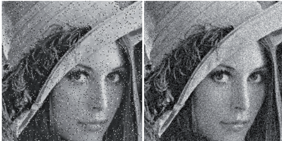
FIGURE 13 Two examples of noisy images: “salt and pepper” noise (on the left) and Gaussian noise (on the right).
