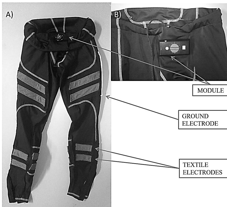
FIGURE 6. The EMG garments (Myontec LTd, Kupio, Finland) measure surface EMG on four muscle groups of lower extremities. A) The front side of the tights and the textile electrodes shown inside out. B) The portable module collecting the data is attached in the front.
