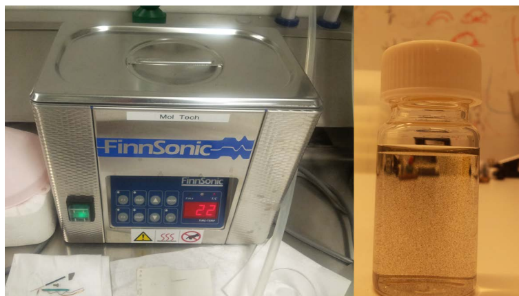
Figure 6.5: (A)FinnSonic sonicator used in the experiment; (B)Dispersed single walled carbon nanotubes in 1,2-dichloroethane
