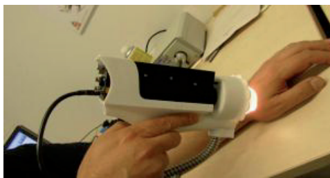
FIGURE 7 Developed hand-held hyperspectral imaging system in use. Image is from Neittaanmäki-Perttu et al. (2013).
