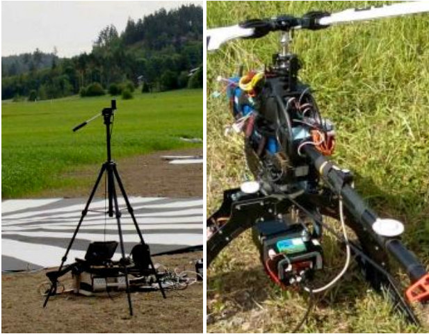
Figure 2. Left, the cosine collector of the ASD FieldSpec pro was placed on a tripod about 1.5 meters from the ground. Right, the FPI spectral camera mounted under a helicopter UAV and the irradiance sensor mounted to the tail boom.
