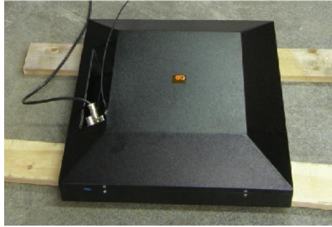
Figure 21: Scintillation detector SC16 (Cropped version of the original photo by Tomi Rähkä)
